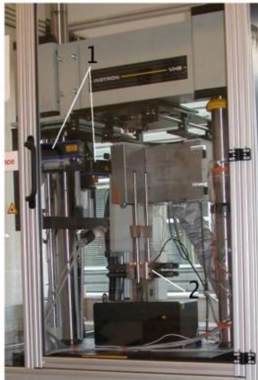
Figure III.9: High-Speed Tensile Testing Device [GAR 08] 1) Doppler-effect laser cells for strain measurement 2) Sample
