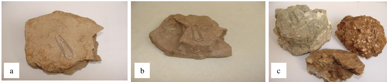
Fig 7 Sampled picked manually from the area, packstone to floatstone (a); marl to lime mudstone (b); gypsum and anhydrite (c)
