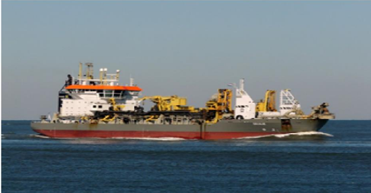
Figure 2. A trailing suction hopper dredge (TSHD) and its primary components for operation.
