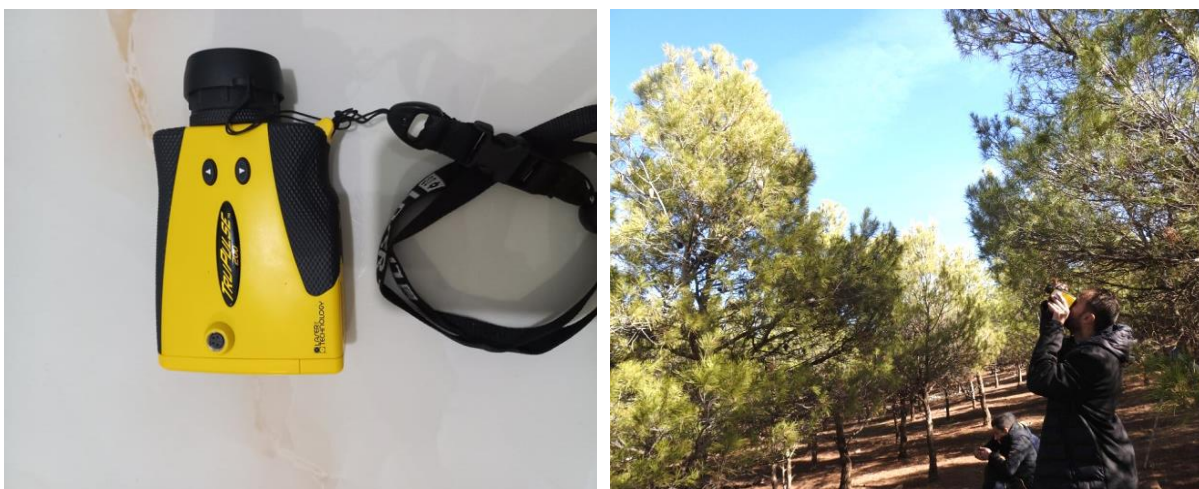
Figure 2. Measuring the height of a Tree with a TruPulse laser rangefinder.
