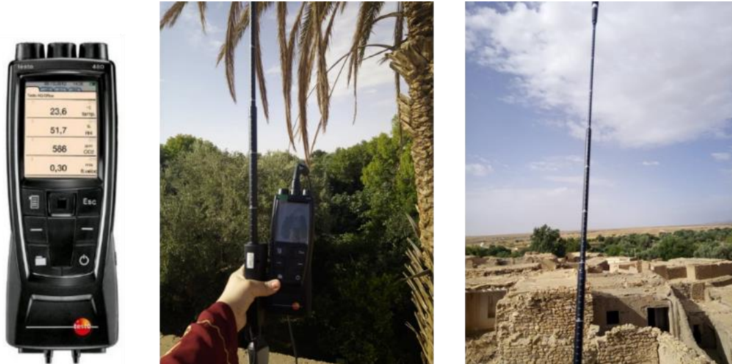
Fig. 7. handheld device Testo 480.
